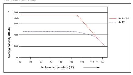
Note: The limit curves for the heat exchangers exchanger apply to a dew point of 149  $^{\circ}$ F.
